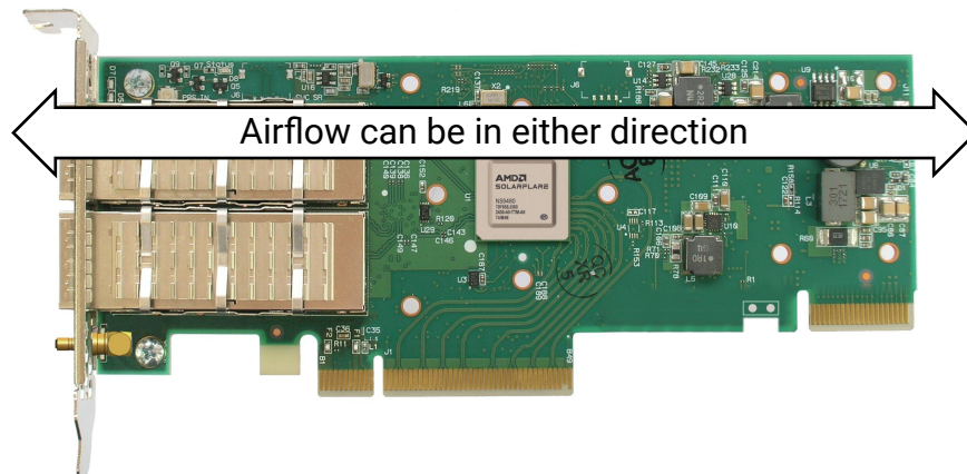
Figure 3: Airflow Direction for X4542 Ethernet Adapters
