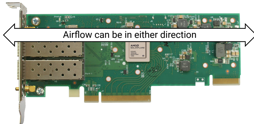
Figure 3: Airflow Direction for X4522 Ethernet Adapters
